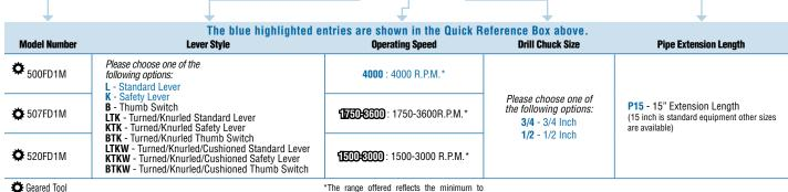
\*The range offered reflects the minimum to maximum operating speeds that this tool can be set. One must choose a speed within this range that best fits the application. Please examine the abrasive used with the tool for a maximum operating speed. The tool should be set at or below the maximum operating speed listed on the abrasive.
