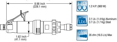
\*Versions 400HGE21M & 400HGE36M add 0.51 Inch (13.0mm) to the overall length. Rear exhaust adds 0.82 Inch (20.8mm) to overall length.
